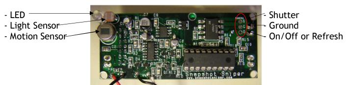
The Snapshot Sniper game camera controller board is the easiest to use, most versatile board available. Below are some of the main features:
