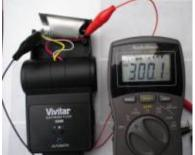
3. Now to modify the 100ohm 10 watt resistor I use a piece of 22 gauge wire. Soldered it to the resistor and covered it with electrical tape. Making a tool that works very well too drain the flash capacitor using this resistor you will see the spark when draining the capacitor and sort of lets you know it has been drained. In the picture I drained it right at the flash tube ends this way I never really expose anything to the high voltage
