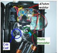
Now we are left to mount the Switch and the battery holder I use a piece of PVC board and attach it to the flash capacitor on the left side with pt1100 tape and on the right side I attach a piece of small plastic angle stock to the case then attach the board to it with PT1100 Tape also. In doing my builds this way I feel it makes a very neat finish with no holes drilled in the case other than the flash hole.
